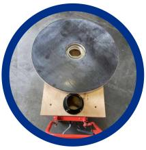
Rotating turn table top for easier prepping and optional vacuum connection to reduce aluminum dust in work area.
