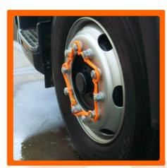
Routine Torque Checking: Simply move the Squirrel sideways using a screwdriver or remove completely and torque in the normal way; then, refit.
