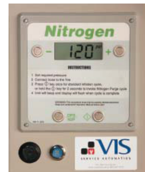
VIS-Nitro automates tire inflation
